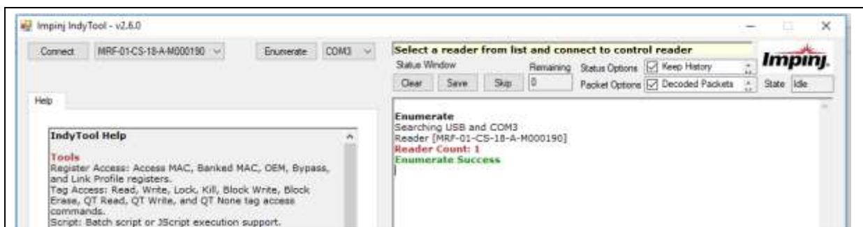
After use, and closing the Reader Application, it is a good idea to disconnect the virtual com port releasing the port. If this is not done, other Applications programs attempting to communicate to the reader may fail.
